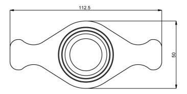
Ball locking ring in rental construction for the use instead of the standard ball locking ring
